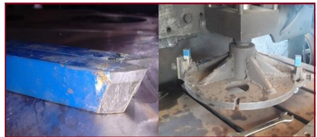
Figure 2 Cutting Tool Holder and single point carbide tip tool
